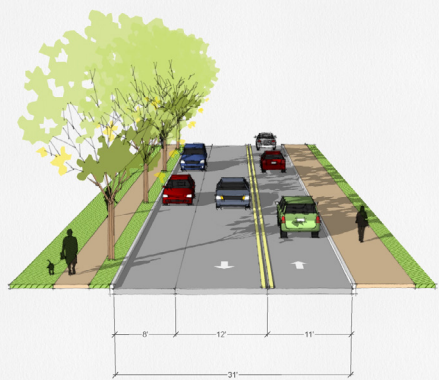
FIGURE 15. EXISTING KANUGA CROSS SECTION
